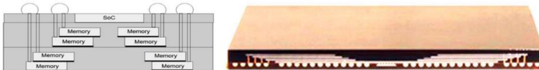
Figure 13. Fan-Out Multi-Stack integration (TSMC MiM). (WLP Chapter Figure 38, and ECTC 2019)
